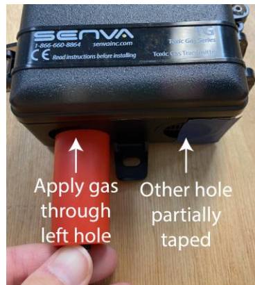
Figure 3: Applying test gas with enclosure closed.
