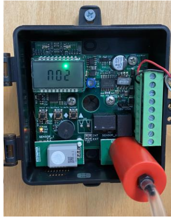
Figure 2: Recommended calibration check setup
